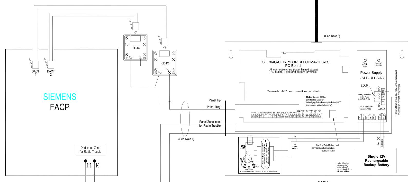
All FACP to radio wiring must be in conduit (20 feet max. for Commercial Fire and 3 feet max. for Residential Fire).
