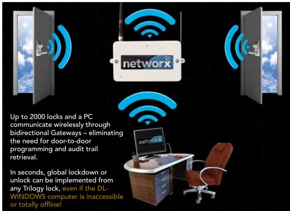
Up to 2000 locks and a PC communicate wirelessly through bidirectional Gateways – eliminating the need for door-to-door programming and audit trail retrieval.
