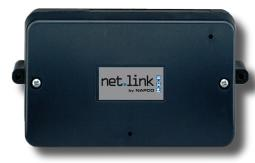
reporting, previously via telephone lines/telco only, can now be communicated over both a TCP/IP network and/or Telco, or via the TCP/IP network as a backup. The NL-MOD module is connected to the on-board serial port of the GEM-X255, GEM-P3200 and GEM-P9600 NAPCO GEMINI Control Panel, or is connected via the bell and PGM wires from the GEM-P1632, GEM-P816, NAPCO Express and other control panels.
