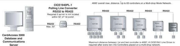
Continental Enterprise Controllers can connect to the server via hardwire (shown above), Ethernet LAN/WAN modem or fiber optics. See the Configuration Guide for additional detailed system information.
