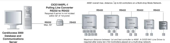
Napco Access Pro Controllers can connect to the server via hardwire (shown above), Ethernet LAN/WAN modem or fiber optics. See the Configuration Guide for additional detailed system information.
