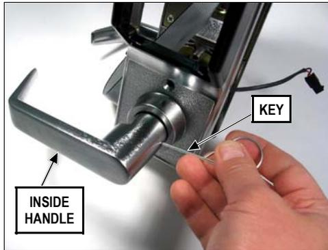
Use key to depress the lever catch pin, then remove the inside handle.
