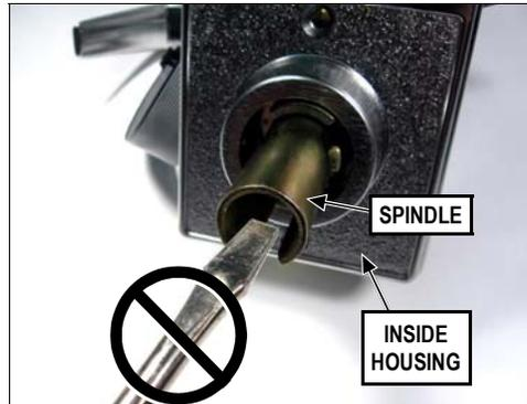
Do NOT insert a screwdriver or other tool into the spindle to release the catch pin, as the catch spring is easily damaged.
